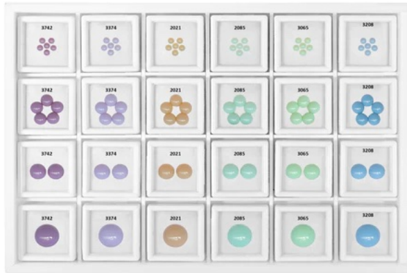
Figure 9. Translucent and Opaque SIAMITE ® . The transparency of cabochons in a row: 3-6-8-12 mm is gradually reduced.
