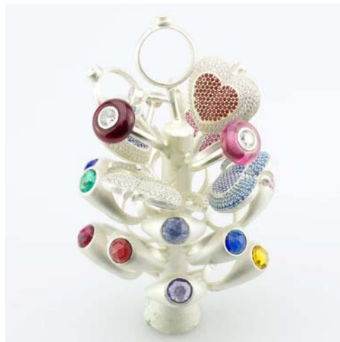
Figure 3. Silver jewelry tree made by the lost wax casting process.
